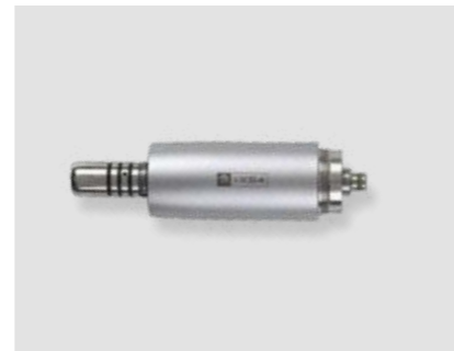
Micromotor i-XS4 The brushless micromotor is integrated with the dental unit electronics, which also controls the peristaltic pump. The software allows precise, safe control of speed and torque (which, with the EVO R20L contra angle, can reach 70 Ncm).
