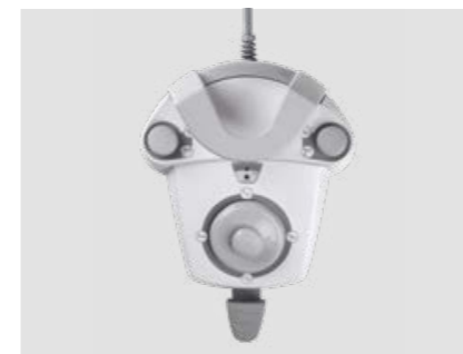
Multifunction Foot Control Cutting-edge device with ergonomic lateral-slide control that lets dentists activate Chip Air and Chip Water functions on the instrument in use, invert micromotor rotation (when extracted), control patient chair movement and recall saved positions.
