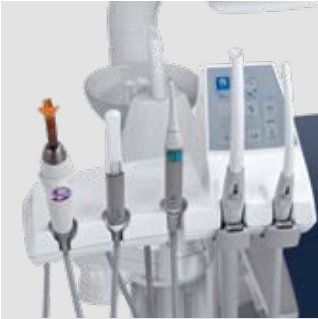
Assistant's module The module mounted on the double-articulated arm is height-adjustable and comes with three holders as standard. An optional 5-holder version is also available: this can be used to hold other instruments such as a video camera or T-LED light. The keypad incorporates controls that move the patient chair, switch on the operating light and operate the water-to-cup and cuspidor bowl rinse functions.
