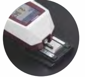
Roughness detector imported from Japan, to test the roughness of metal surface
